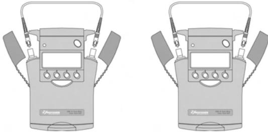
34. On both instruments: switch on, set [AUTOTEST], and warm up for a few minutes.
