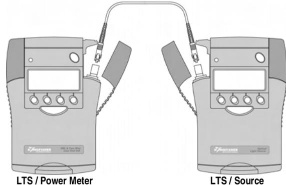
Test set-up for both the Output Power and Short Term Stability Tests
