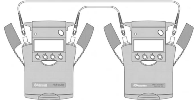
Simultaneous one way loss testing
