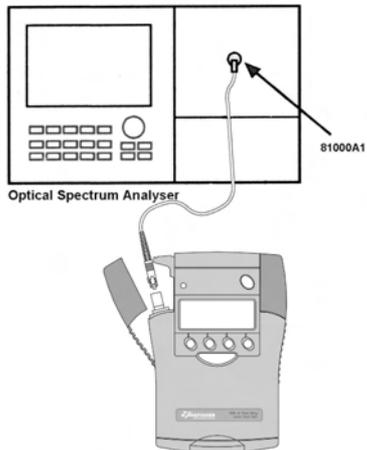
Test set-up for the centre  $\lambda$  and spectral bandwidth
